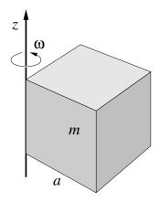
(CM3) A cube of mass m has constant density and edge length a. The cube rotates about a fixed axis (z) on one edge, at fixed angular frequency  $\omega$ .
