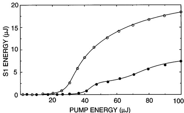
Fig. 2. Dependence of the energy of the first Stokes component (S1) on the energy of the pump pulses. Filled circles, S1 without seed; open circles, S1 with seed. The seed pulse energy is  $10^{-6}$   $\mu\text{J}$ .
