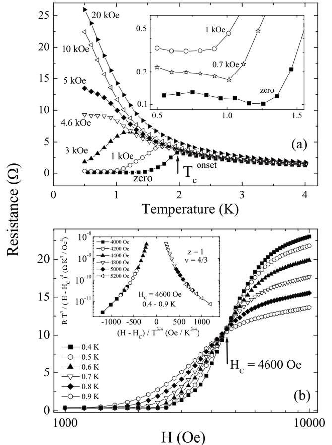
FIG. 4. (a)  $R(T)$  in magnetic field for sample displaying metallic behavior below  $T_c^{\text{onset}}$ . The inset highlights metallic behavior at low  $H$ . (b) Isotherms showing  $H_c = 4600$  Oe. The inset shows data collapse near  $H_c$  by using two-parameter scaling (Ref. 21).
