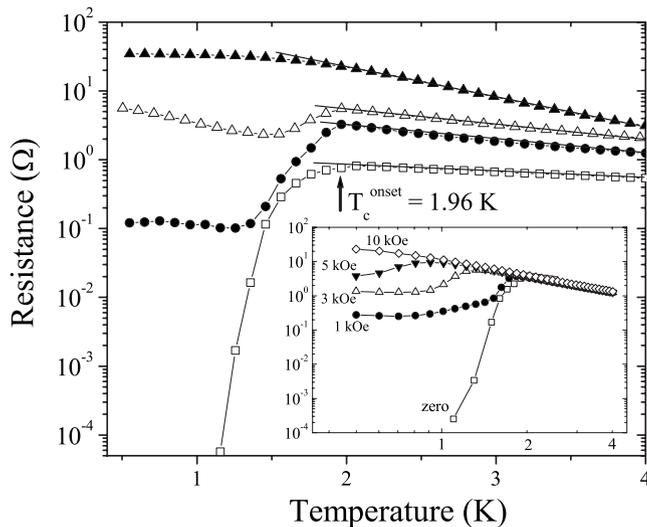
FIG. 3.  $R(T)$  for four as-grown (i.e., no annealing) crystals showing disorder-induced metallic state below  $T_c^{\text{onset}}$ . The inset shows sample of main panel (open squares) in magnetic field.
