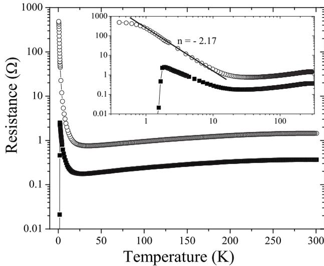
FIG. 2. Electrical resistance for superconducting and nonsuperconducting crystals. *Insulating* behavior was induced through 10 h anneal of a superconducting crystal in air at 200 °C. The metallic regimes above  $T_M$  have similar  $\alpha_a$  values. The inset shows a log-log scale and fit to Eq. (3).
