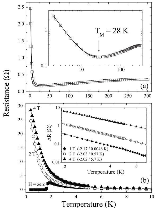
FIG. 1. (a) Electrical resistance for a typical  $\text{Li}_{0.9}\text{Mo}_6\text{O}_{17}$  crystal. The inset shows a log-log scale. Lines are fits [Eq. (2) with  $T_0=0$ ].  $T_M=28$  K separates *metallic* and *insulating* behaviors. (b) Data for  $H \leq 4$  T. The inset compares to 1D hopping mechanism [Eq. (3)]. Numbers in parentheses are  $n$  and  $T_0$ .
