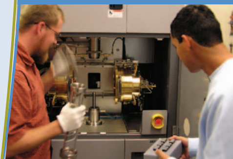
Students and postdocs work with MSU's optical-image furnace to grow single crystals of advanced materials
